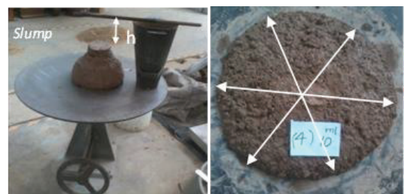
Figure 1 - Workability Test Procedure
