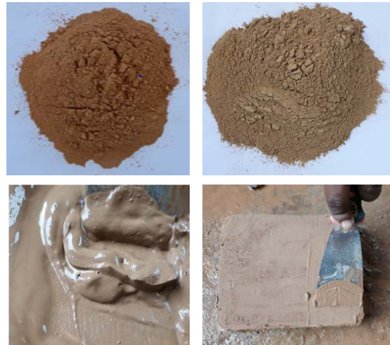
Fig. 4. Prepared clay cement mix and application process
