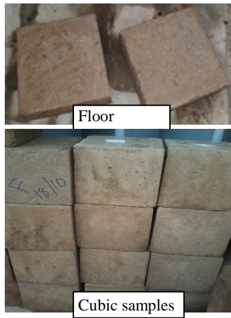
Fig. 2. Prepared floor sample and cubical samples
