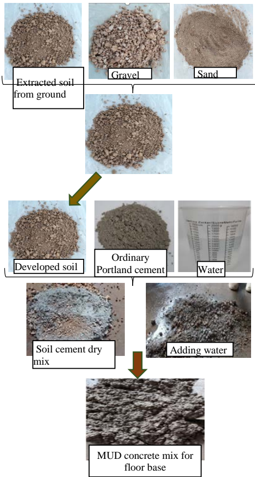
Fig. 1. Mud concrete preparation process
