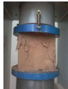
Fig. 10. Compressive strength test procedure
