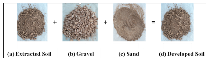
Fig. 2. Existing soil preparation to required composition
