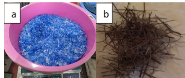
Figure 2: (a) Shredded polyethylene and (b) pieces of Kithul
