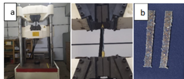
Figure 6: (a) Tensile test equipment and (b) Tensile samples
