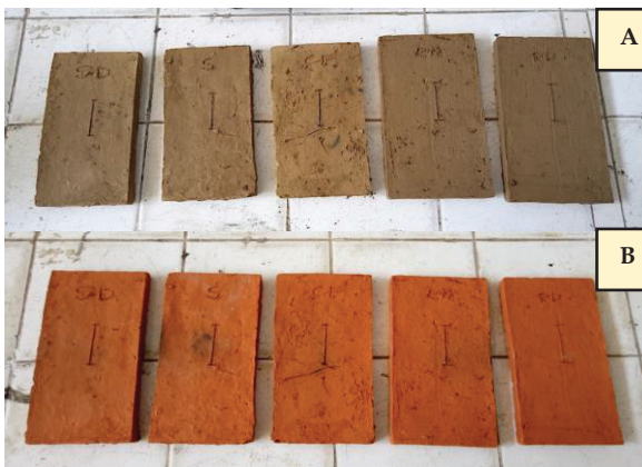
Figure 7 - Red Clay Panels Mixed with Different Compounds - (A) Before Firing and (B) After
